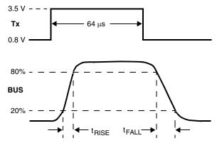
Figure 5. BUS Rise and Fall Times
