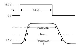
Figure 6. Pulse Width Distortion
