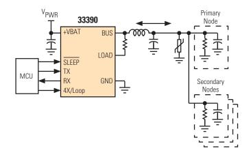
Figure 1. 33390 Simplified Application Diagram
