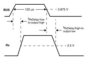
Figure 8. BUS-to-Rx Delay Time
