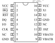
16-PIN DIP (300 MIL) 16-PIN SO (300 MIL) 16-PIN SSOP (208 MIL) See Mechanical Drawings Section
