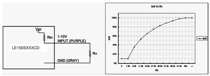
**Dimming Configuration using External Resistance**
