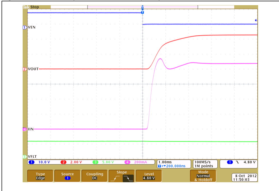
Figure 18. Soft-start performance for 100 \mu\text{F} capacitive load
