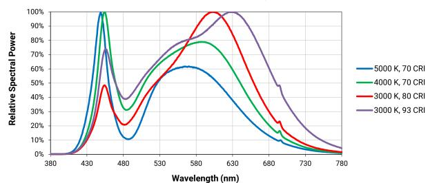
The following graph is the result of a series of pulsed measurements at 1900 mA and  $T_J$  = 85 °C.
