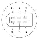
Pin assignment plug FireWire
