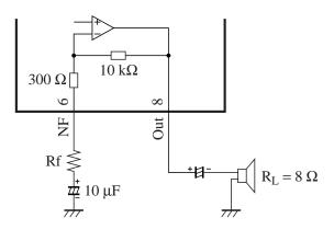
Bass boost can be easily implemented by inserting a series connection of RC between Pin8 (output) and Pin6 (NF). Example :  $Rb = 12 k\Omega$ ,  $Cb = 0.022 \mu F$
