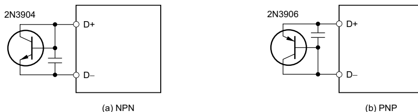
Figure 88. Remote Temperature Sensor Using Transistor
