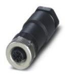
Connector, 4-position, Socket straight M12, S-coded, Screw connection, Knurl material: Zinc die-cast, nickel-plated, Cable gland Pg11, External cable diameter 8 mm ... 10 mm
