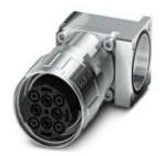
Device connector, front mounting with knurled nut, angled fixed, SPEEDCON locking, M40, Number of positions: 2+3+PE, Type of contact: Socket, Crimp connection, Axial O-ring, 4x Ø4,2, Shielded: Yes, Flange dimensions: 40 mm x 40 mm
