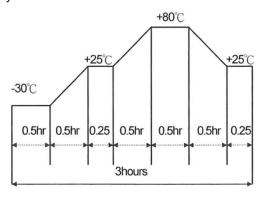
The diaphragm will be measured after being placed at  $+25^{\circ}$ C for 4 hours. The value of the resonant frequency should be  $\pm 10\%$ , the value of the electro static capacitance should be  $\pm 20\%$  compared to the initial measurements. The resonant impedance should be  $2,000~\Omega$  max.
