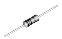
A metal glazed film is deposited on a high grade ceramic body. After that caps are applied to the rods and tinned electrolytic copper wires are welded to these end caps. The resistors are coated with a light-blue lacquer which provides electrical, mechanical and climatic protection. The encapsulation is resistant to all cleaning solvents according to IEC 60068-2-45.
