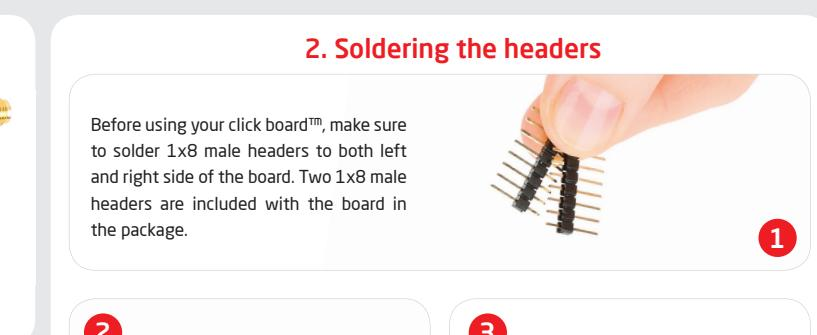
Before using your click board™, make sure to solder 1x8 male headers to both left and right side of the board. Two 1x8 male headers are included with the board in the package.
