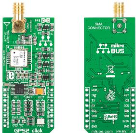
GPS2 Click™ is an accessory board in **mikroBUS™** form factor. It's a compact and easy solution for adding GPS module to your design. It features **Quectel L30** GPS module as well as SMA antenna connector. GPS2 Click™ communicates with target board microcontroller via **mikroBUS™** UART (Tx, Rx), I<sup>2</sup>C (SCL, SDA), SPI (MISO, MOSI, SCK, CS), PWM, INT, AN and RST lines. The board is designed to use 3.3V and 5V power supply. LED diode (GREEN) indicates the presence of power supply.
