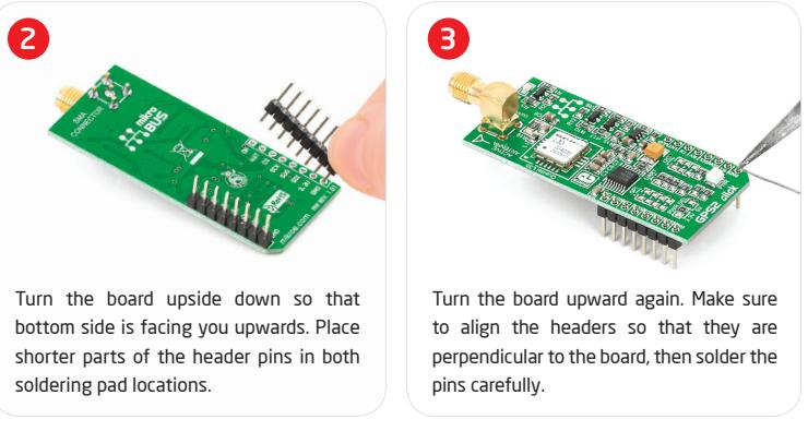
Turn the board upside down so that bottom side is facing you upwards. Place shorter parts of the header pins in both soldering pad locations.
