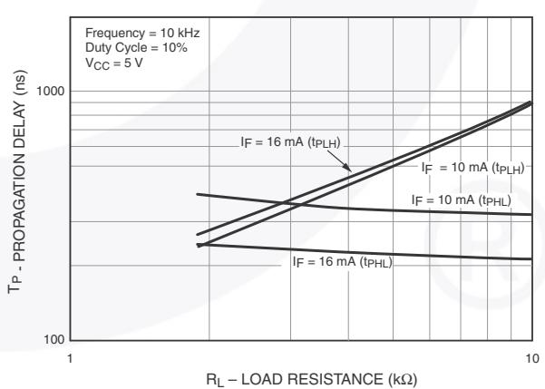
Figure 8. Propagation Delay vs. Load Resistance
