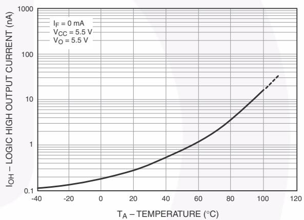
Figure 12. Logic High Output Current vs. Temperature
