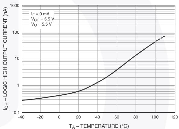
Figure 6. Logic High Output Current vs. Temperature
