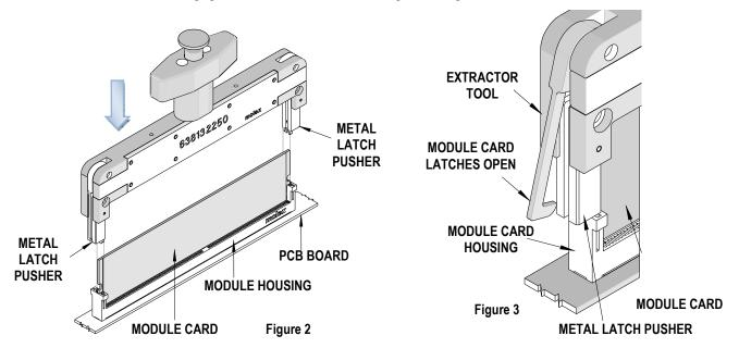
3. Make sure the extractor tool is firmly seated in the slots of the module card housing and the module card latches are locked into the module card.
