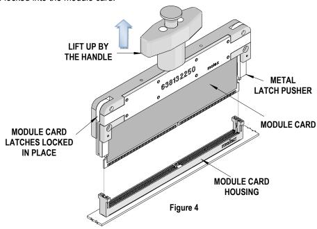
4. Pull the module card straight up with the handle of the extractor tool. See Figure 4.
