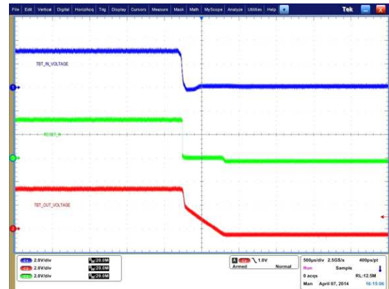
Figure 15. TBT_OUT Load Transient Response (3.5A to 0.5A Step)
