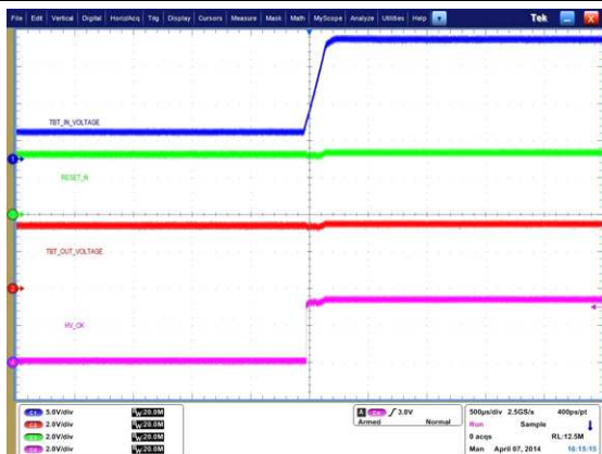
Figure 16. 0V to 3.3V Power Up With 50mA Load
