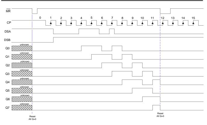
Notes: 5. All Q values are reset to LOW when  $\overline{MR}$  goes low.  $\overline{MR}$  is asynchronous and overrides all other signals.
