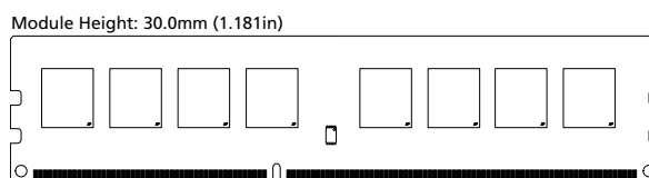
Figure 2: 240-Pin UDIMM (MO-269 R/C-A1)
