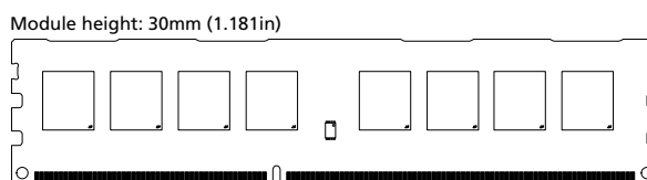
Figure 2: 240-Pin UDIMM (MO-269 R/C-A1)
