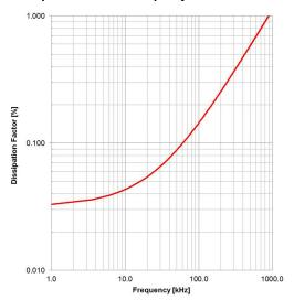
Test Equipment: E4991A or equivalent
