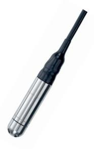
The ILS is designed for use in continuous submersion in liquids such as water, oil and other non-aggressive chemicals. The submersible uses the latest piezo-resistive media-isolated silicon sensing technology and a stainless steel diaphragm within a 316L stainless steel housing.
