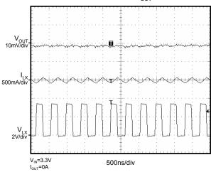
Output Voltage Ripple ( $V_{OUT}$ =1.5V)
