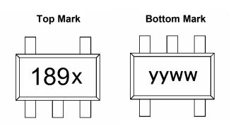
Marking for SOT23, 5 Lead Package: x = Code of the output voltage (Example: C for VOUT=1.20V) yyww = Datecode (Example: 0852)
