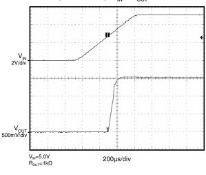
Start Up (Power up  $V_{IN}$ ) ( $V_{OUT}$ =1.5V)
