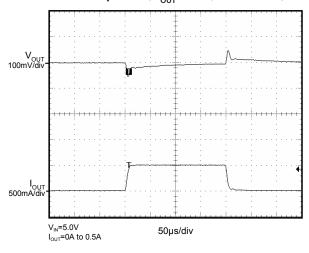
Transient Response (V<sub>OUT</sub>=3.3V; 0.5A to 1.0A)
