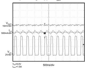
Output Voltage Ripple (V<sub>OUT</sub>=1.5V)
