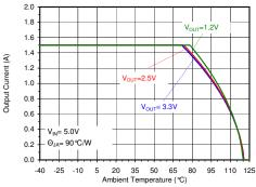
Figure 3 — Typical maximum output current over temperature of SOT23-5 package, V<sub>IN</sub>= 5.0V
