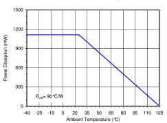
Figure 2 — Maximum power dissiption of SOT23-5 package over temperature
