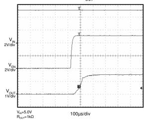
Start Up (Enable)(V<sub>OUT</sub>=1.5V)
