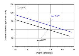
Figure 5 — Current limit holding current decreasing rate vs. output voltage
