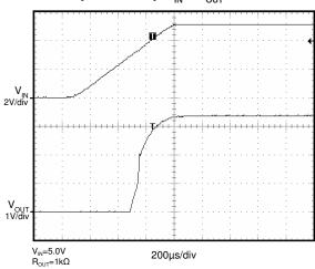
Start Up (Power up  $V_{IN}$ ) ( $V_{OUT}$ =3.3V)
