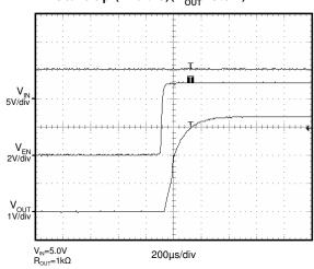
Start Up (Enable)(V<sub>OUT</sub>=3.3V)
