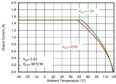
Figure 4 — Typical maximum output current over temperature of SOT23-5 package, V<sub>IN</sub>= 3.3V
