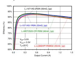
Figure 6 — Typical efficiency curves  $(V_{IN}=5.0V, V_{OUT}=3.3V)$
