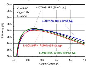
Efficiency vs. Load Current (SOT23-5)
