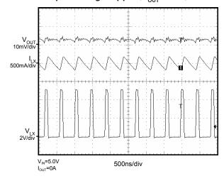
Output Voltage Ripple (V<sub>OUT</sub>=1.0V)
