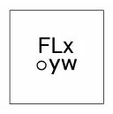
Marking for 2mm x 2mm MLPD-UT 6 Lead Package: x = Code of the output voltage (Example: C for VOUT=1.20V) oyw = Pin 1 and Datecode (Reference Package Marking Design Guidelines, Appendix A)
