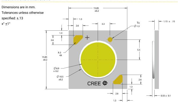
Datasheet of CXB1512-0000-000N0HM427G - LED ARRAY 9MM 2700K 80CRI 1485LM Contact us: sales@integrated-circuit.com Website: www.integrated-circuit.com
