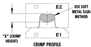
Use soft metal slug (solder) method to measure the "X" dimension. Verify tooling crimp height calibration by referring to the Go/No Go dimensions shown in the chart below.
