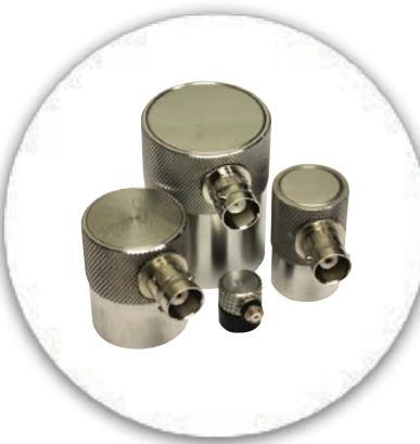
Contact Transducers are the most common and frequently used to introduce longitudinal waves into a material. Also, by using special elements, normal incidence shear wave or a combination of longitudinal/shear wave transducers can be made. These types of transducers are used in direct contact with the test material and therefore require a highly durable wearplate.
