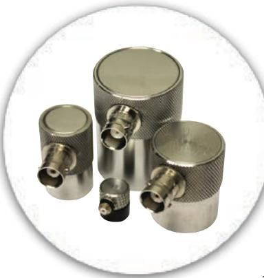
Shear Wave Transducers are designed to excite shear waves directly into a material without the use of angle beam wedges. Unique design parameters have been incorporated to minimize the longitudinal component. Applications include direct shear wave velocity, Young's modulus of elasticity and shear measurements. The shear direction on all transducers is parallel to the right angle connector unless otherwise specified. Special longitudinal/shear combinations are available in a single transducer.
