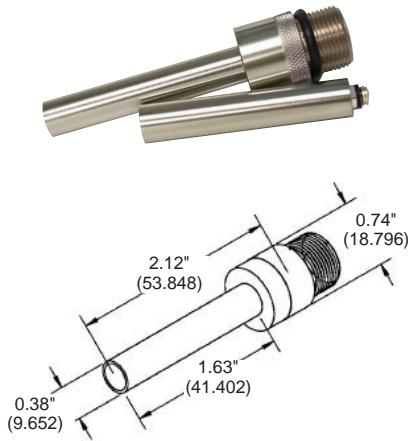
Pencil Case Style Immersion Transducers combine small case diameters and extended working length facilitating access where hard to reach areas are encountered. These Pencil Case Styles are offered in P style (UHF connector) and an PM style (microdot connector) with element diameters of 0.125" and 0.250". Both spherical and cylindrical focal lengths are available as options.
