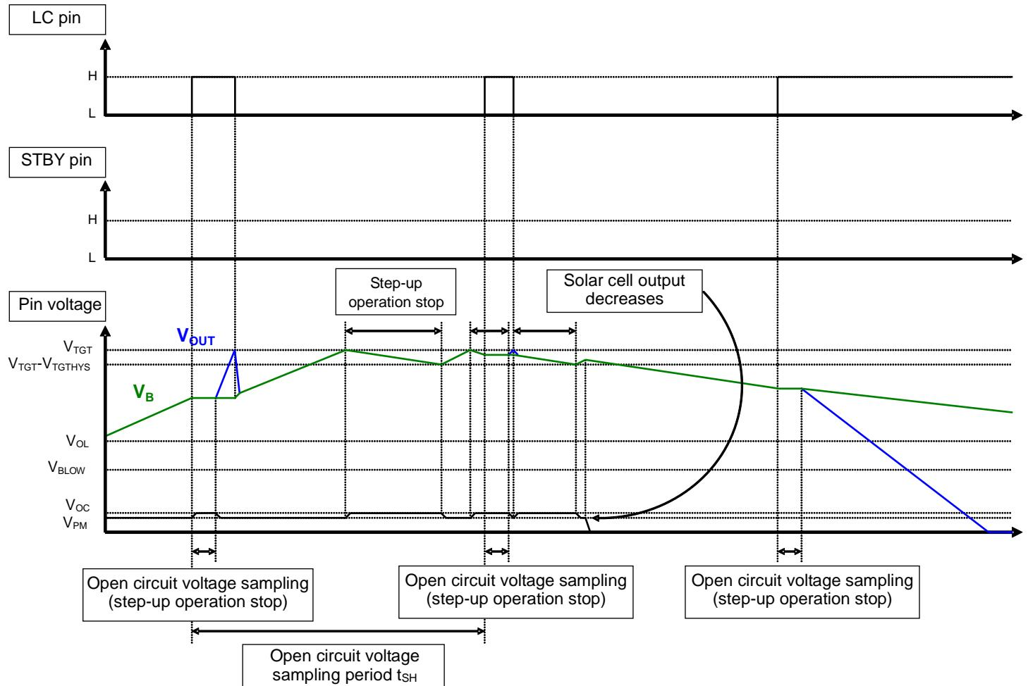
Figure 3. Behavior of when solar cell output decreases
