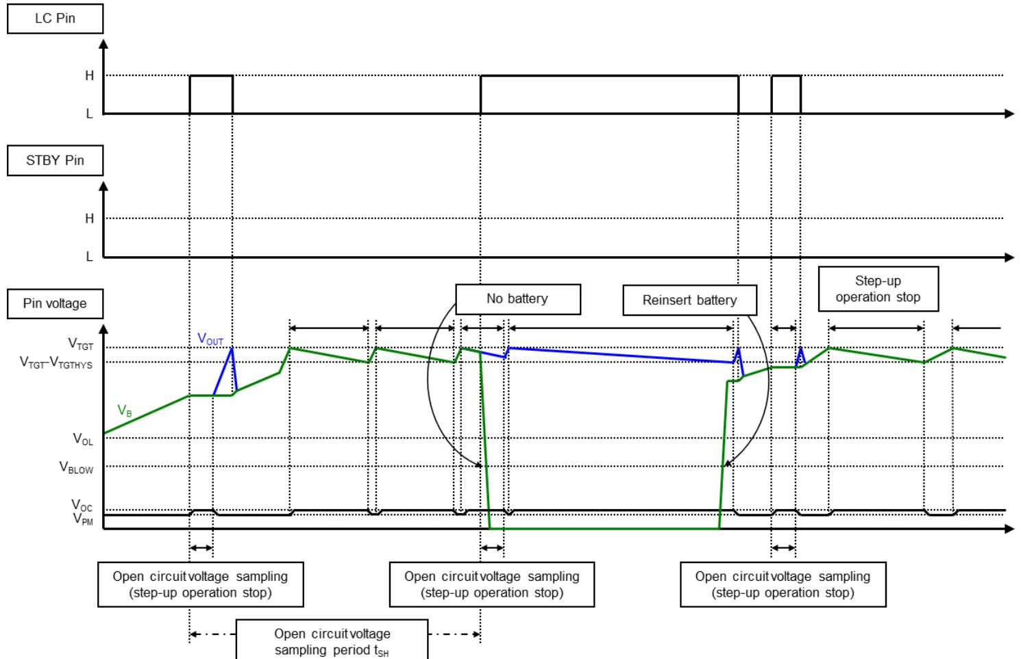
Figure 5. Behavior of when no battery is connected.
