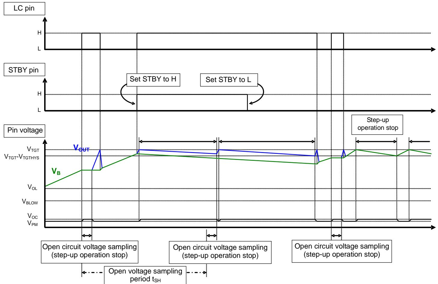
Figure 4. Behavior when the STBY pin is asserted
