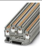
Double-level terminal block, Cross section: 0.14 mm² - 4 mm², AWG: 26 - 12, Connection type: Push-in connection, Width: 5.2 mm, Color: orange, Mounting type: NS 35/7,5, NS 35/15
