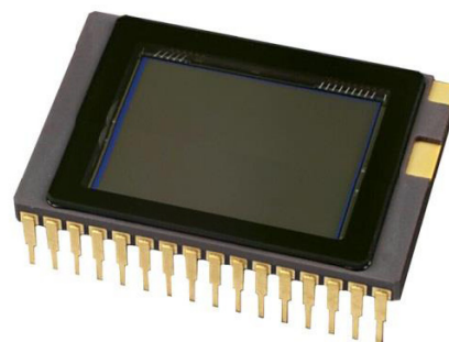
Figure 1. KAF-8300 Full Frame CCD Image Sensor
