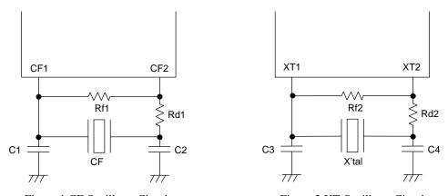
Figure 1 CF Oscillator Circuit
