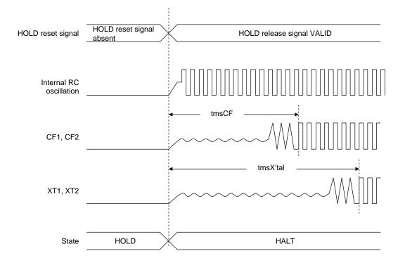
HOLD Reset Signal and Oscillation Stabilization Time
