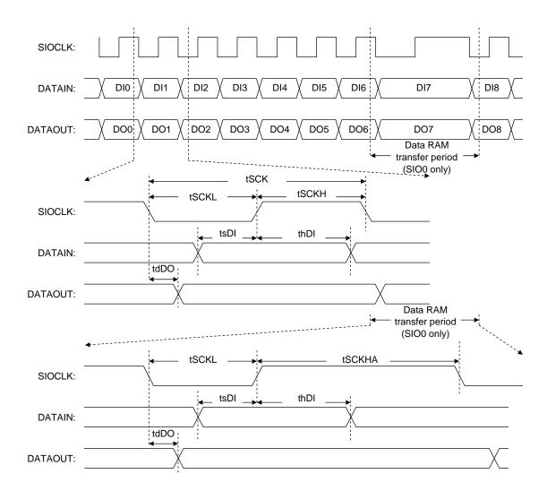
Figure 6 Serial I/O Waveforms
