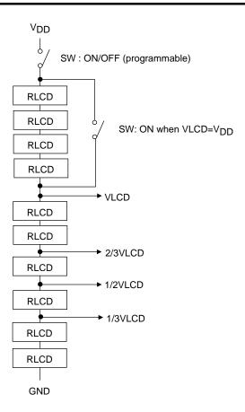
Figure 8 LCD Bias Resistors
