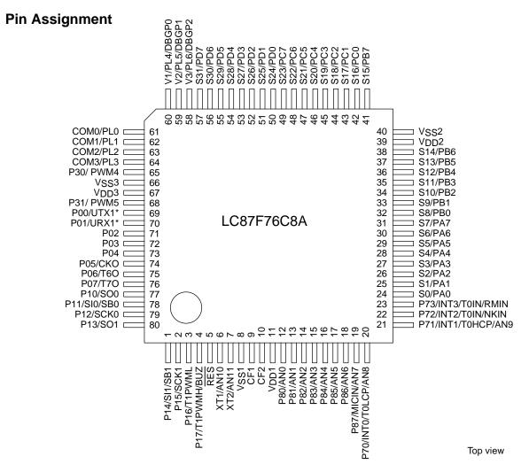
\*When using UART, set P0LDDR (PODDR: Bit0) to "0" SANYO: QFP80(14×14) "Lead-free Type" SANYO: TQFP80J(12×12) "Lead-free Type"
