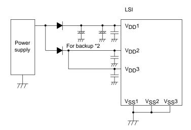
\*2 The internal memory is sustained by V<sub>DD</sub>1. If none of V<sub>DD</sub>2 and V<sub>DD</sub>3 are backed up, the high level output at the ports are unstable in the HOLD backup mode, allowing through current to flow into the input buffer and thus shortening the backup time.
