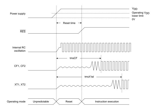
Reset Time and Oscillation Stabilization Time
