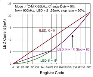
Figure 5. LED Current vs. Register Code
