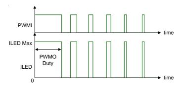
Figure 1. PWM Dimming
