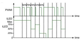
Figure 3. Mixed Mode Dimming
