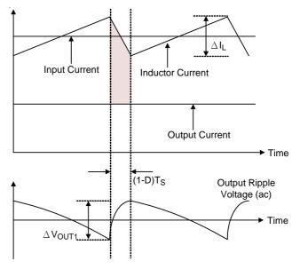
Figure 14. The Output Ripple Voltage without the Contribution of ESR
