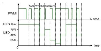
Figure 2. DC Dimming
