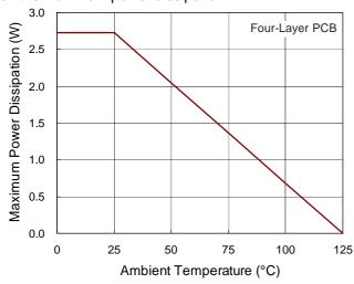
Figure 15. Derating Curve of Maximum Power Dissipation
