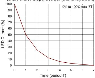
Figure 11. LED Current (Dimming Down) vs. Time
