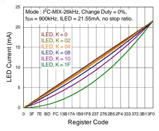
Figure 4. LED Current (Different Compensation Ratio) vs.
