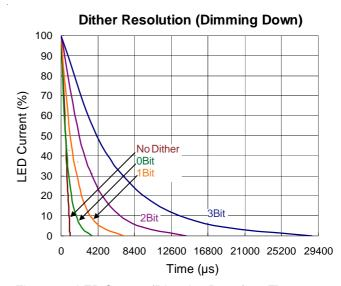
Figuer 13. LED Current (Dimming Down) vs. Time
