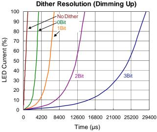
Figuer 12. LED Current (Dimming Up) vs. Time
