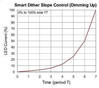
Figure 10. LED Current (Dimming Up) vs. Time
