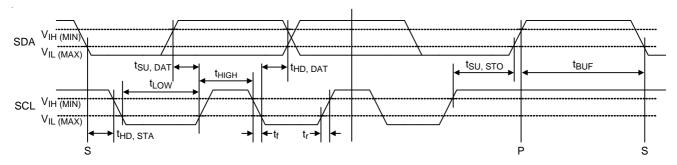
RT8555  $I^2C$  slave address = 7'b0110\_001.  $I^2C$  interface support fast mode (bit rate up to 400kb/s). The write or read bit stream (N  $\geq$  1) is shown below
