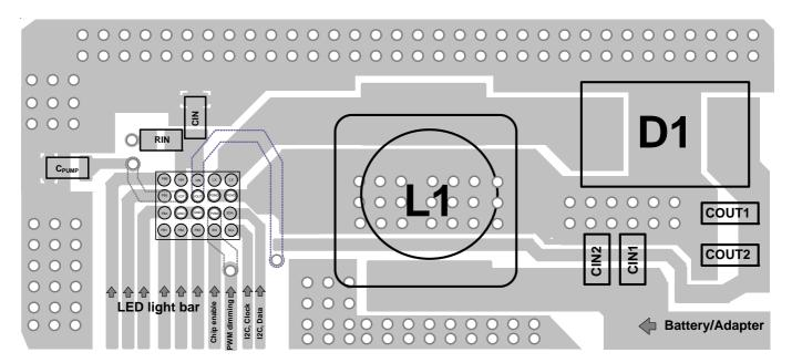
Figure 16. PCB Layout Guide
