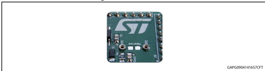
Figure 4: Mounting through-hole sense resistor
