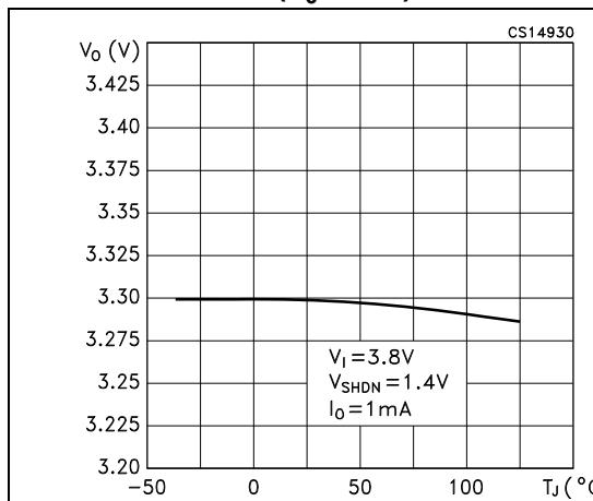
**Figure 7. Shutdown voltage vs. temperature
