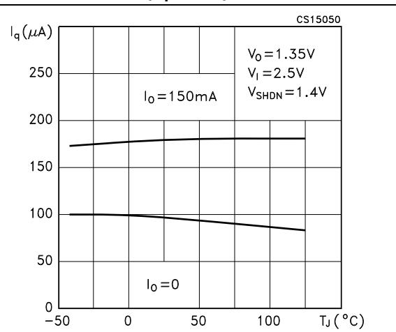
**Figure 16. Quiescent current vs. temperature ( $V_l=6$  V)**
