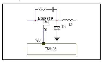
The RC components should realise a time constant corresponding to one tenth of the switching time constant of the TSM108 (i.e. in our example, the oscillator frequency is set to  $10\mu$ s corresponding to 100kHz, therefore, the RC couple should realise a time constant close to  $1\mu$ s).
