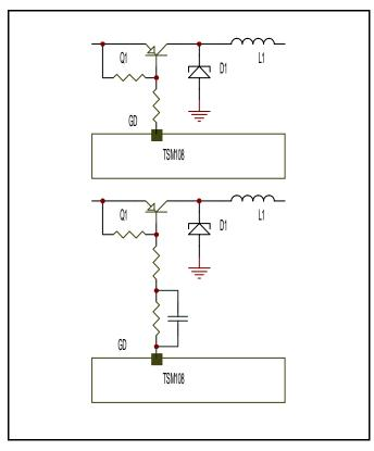
The most immediate way to choose between a P-channel MOSFET or a PNP transistor is to consider the ratio between the output power of the application and the expected components price: the lower the power, the more suitable the PNP transistor is; the higher the power, the more suitable the P-channel MOSFET is. As an example, for a DC/DC adaptor built for 12V/6V, the recommended limit to choose between P-channel Mosfet and PNP transistor is around 200mA.
