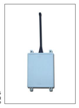
Each Rx decoder incorporates an 'easy learn' feature enabling it to learn the Transmitter encoder signature code as it is transmitted. Each 008 decoder is able to learn up to 50 individual Transmitter encoders (memorised even if the power is removed).
