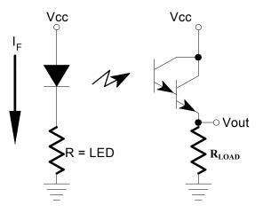
The light source is a pulsed LED with a rise time of less than 500 nS. The LED output is adjusted for  $I_{C} = 0.8$  mA.
