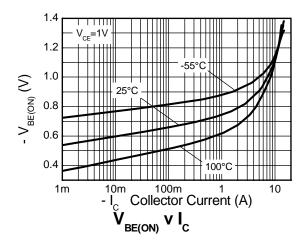
Datasheet of ZXT951KTC - TRANS PNP 60V 6A D-PAK
