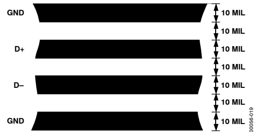
Figure 19. Arrangement of Signal Tracks
