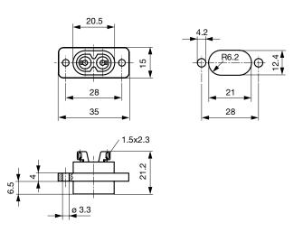
Solder terminals for wires
