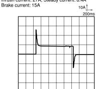
6-(2). Electrical life test (Motor lock) Sample: CF2-12V, 3pcs. Load: 20A 14V DC,
