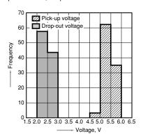
5. Distribution of operate and release time Sample: CF2-12V, 100pcs. With diode
