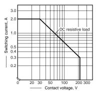
4. Electrical life (2A 30V DC resistive load) Tested sample: TX2-5V, 6 pcs. Operating speed: 20 cpm
