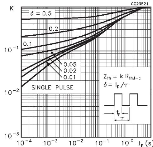
Thermal Impedance For D2PAK / PowerSO-10
