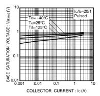
Fig.3 Base-emitter saturation voltage vs. Collector Current
