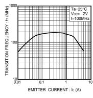
Fig.6 Gain Bandwidth Product vs. Emitter Current
