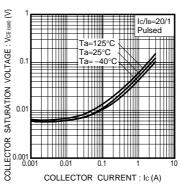
Fig.2 Collector-Emitter Saturation Voltage vs. Collector Current
