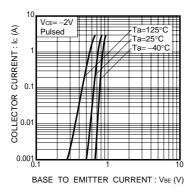
Fig.4 Grounded Emitter Propagation Characteristics
