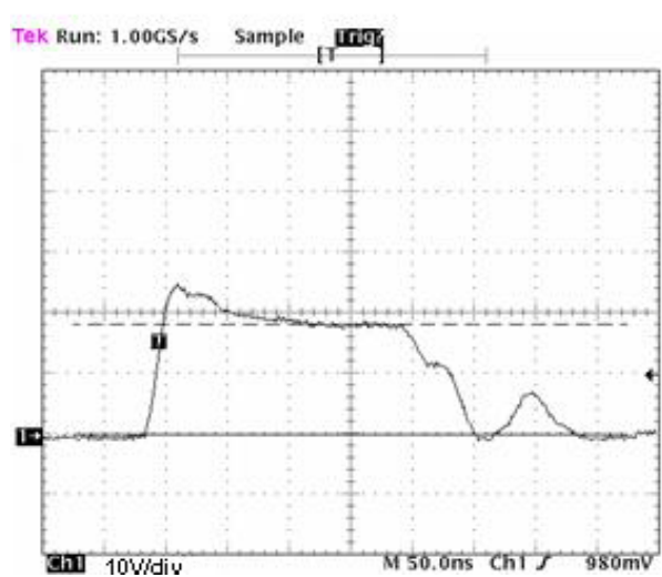
Figure 6. SMS15CT1 ESD Response for IEC 61000-4-2 (+8.0 kV Contact)
