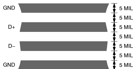
Figure 28. Arrangement of Signal Tracks
