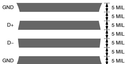
Figure 28. Arrangement of Signal Tracks
