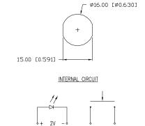
\*UNLESS OTHERWISE SPECIFED TOLERANCES PER DECIMAL PRECISION ARE: X=±1 (±0.039), X,X=±0.5 (±0.020), X,XX=±0.25 (±0.010), X,XXX=±0.127 (±0.005). LEAD SIZE=±0.05 (±0.002), LEAD LENGTH=±0.75 (±0.030). MIN: +DECIMAL PRECISION MAX:= +DECIMAL PRECISION
