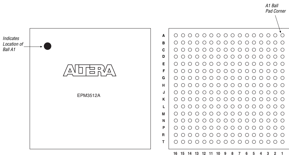
Figure 18. 256-Pin FineLine BGA Package Pin-Out Diagram
