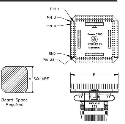
The patented locking mechanism holds the clip on the device by gripping the chip body at the end of each lead pattern. Each contact is individually cantilevered to assure positive contact. Three other types of interfaces are available for connection to your instruments. See Pomona's full line catalog for complete details. Other clips are available in many sizes to fit the most popular chips now in use.
