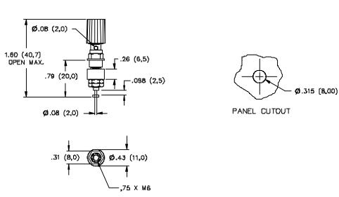
Recommended Maximuml Panel Thickness: .12" (3,0mm)
