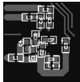
Figure 28. Silkscreen and Bottom Layer Routing
