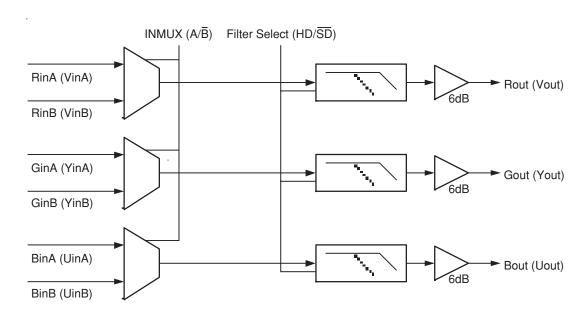
Datasheet of FMS6418AM16X - IC DRVR VID TRPL SEL FLTR 16SOIC Contact us: sales@integrated-circuit.com Website: www.integrated-circuit.com
